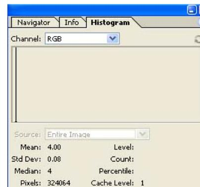
The histogram on left is a typical example of a GEViCAM B/W camera at factory default. The Std Dev of 0.08 translates to 70 dB over 324000 pixels!
