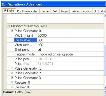
The delay is pulse state low and width is high. For pulse width control the camera responds to low period as the exposure control and the total cycle as the trigger duration. In the example, granularity is 3 µs
