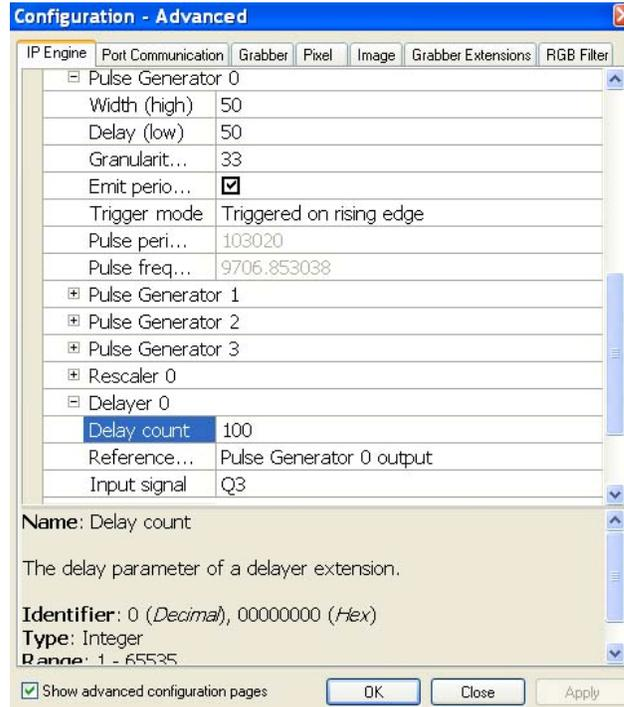
Also in Pulse Generator 0, set periodic and clock frequency. In this example, we set granularity to 33 to make 1µs pulse duration at minimum and Width and Delay for 50 each making 1 cycle of 100 counts (=100µs = 10KHz). Then, Delayer generates delays of 100µs per count. Above picture is set fort 100 delay counts (100x100µs= 10ms).
