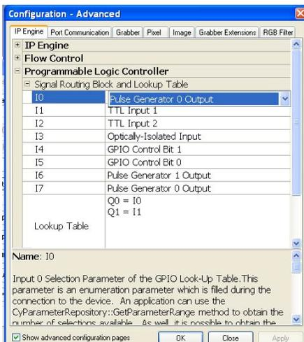
One of the most versatile applications is using the pulse width control function. To do this software triggering, we use pulse generator 0 of Enhanced Function block. First, we set LUT as follows,
