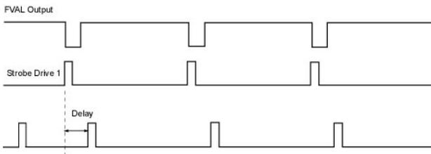
(Note: Strobe drive signal must be generated externally using falling edge of FVAL pulses.)
