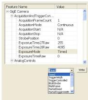
With external trigger input (TTL as default), these ad vanced functions are controllable from MIL. The most common functions are; Exposure-TimeRaw (shutter speed control by increment of 1H), GainRaw(gain control up to 42 dB), and Gamma/Linear selection. The color data is output as individual raw pixel data.
