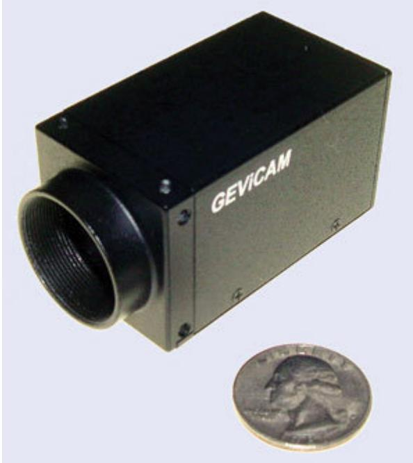
*One of the smallest GigE cameras on the market, the GEViCAM VGA-based camera measures 34 x 34 x 60 mm. Future versions will incorporate a neural-network-based image processor in the package.*
